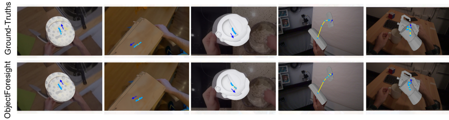
Fig. 5: Qualitative results from ObjectForesight. From the left, the first three columns are from the curated dataset from EpicKitchen and the final two columns are from the HOT3D-Clips dataset. For each sequence, we overlay 8 predicted poses on the last observed frame, illustrating the projected object centers, the transformed object mesh, and the general direction of the movement using an arrow. The images are zoomed in for clarity.
